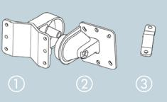
Screw the connector flange (2) to the back of the housing with the four screws and their washers.
